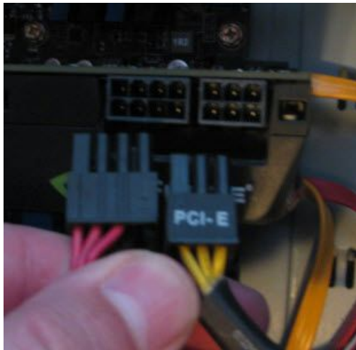
Fig. 8b: Attach Power Cables to Video Card
