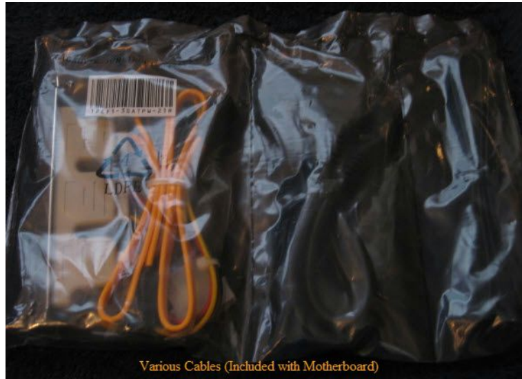
Fig. 1c: Assortment of Cables Included with Motherboard (SATA cables are yellow)
