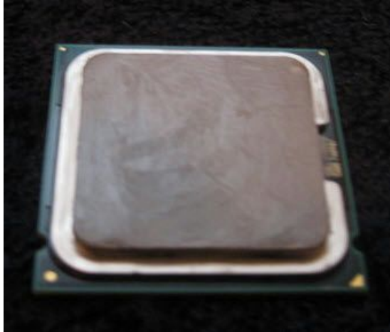
Fig. 2d: Thermal Compound Spread Evenly over Surface of CPU
