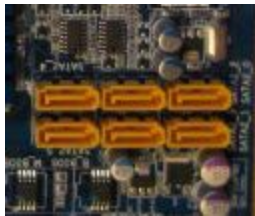
Fig. 10a: Typical SATA Array on Motherboard
