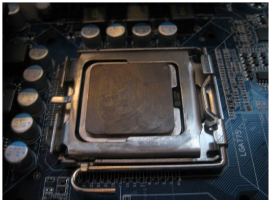
Fig. 3b: CPU Secured in Motherboard Socket
