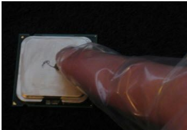
Fig. 2c: Spreading Compound with Plastic Bag over Finger
